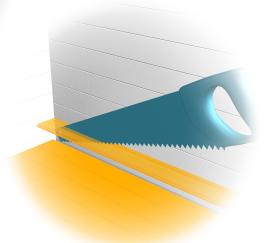
LEAVE 3MM GAP BETWEEN THE BOARDS. SAW THE BOARDS IF NEEDED. 87%
