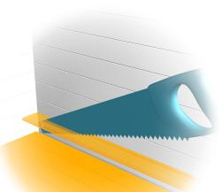
KOLDING 40 SAW THE BASEBOARDS AND ATTACH WITH NAILS AT EVERY 0,5 METERS. ×4, × 35 **\$**BB 85%
