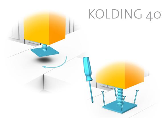
USE SCREWS TO ATTACH THE POST FOOT TO THE HANDRAIL. 40%
